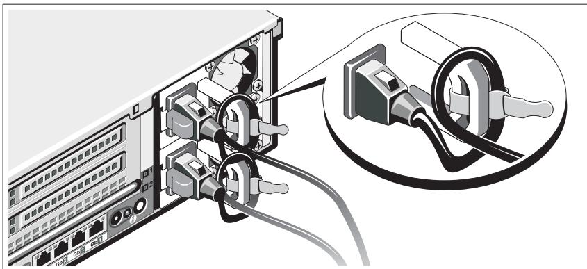
Attach the power cable retention bracket on the right bend of the power supply handle. Bend the system power cable into a loop as shown in the illustration and attach to the bracket's cable clasp.
